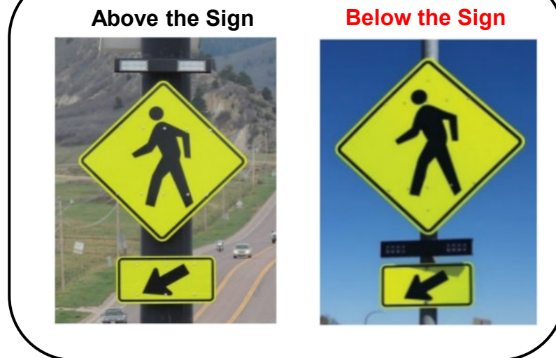
Evaluation of effectiveness based on the relative position of the beacon and the sign (Fitzpatrick, 2016)
